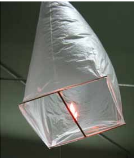
Step 10: Flight! Watch the balloon carefully as it flies and extinguish the fire before it reaches the wood frame.
